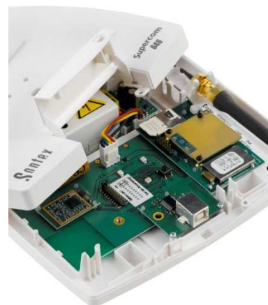
Supercom 646, main power supply 230 VAC, USB, GPRS
