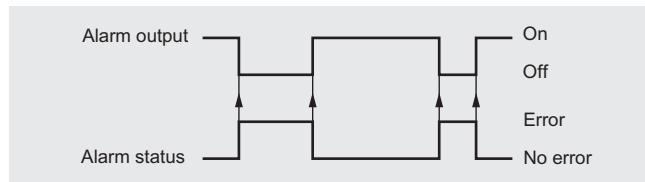
Pulse output B can be used as stated above or as alarm or call up function
