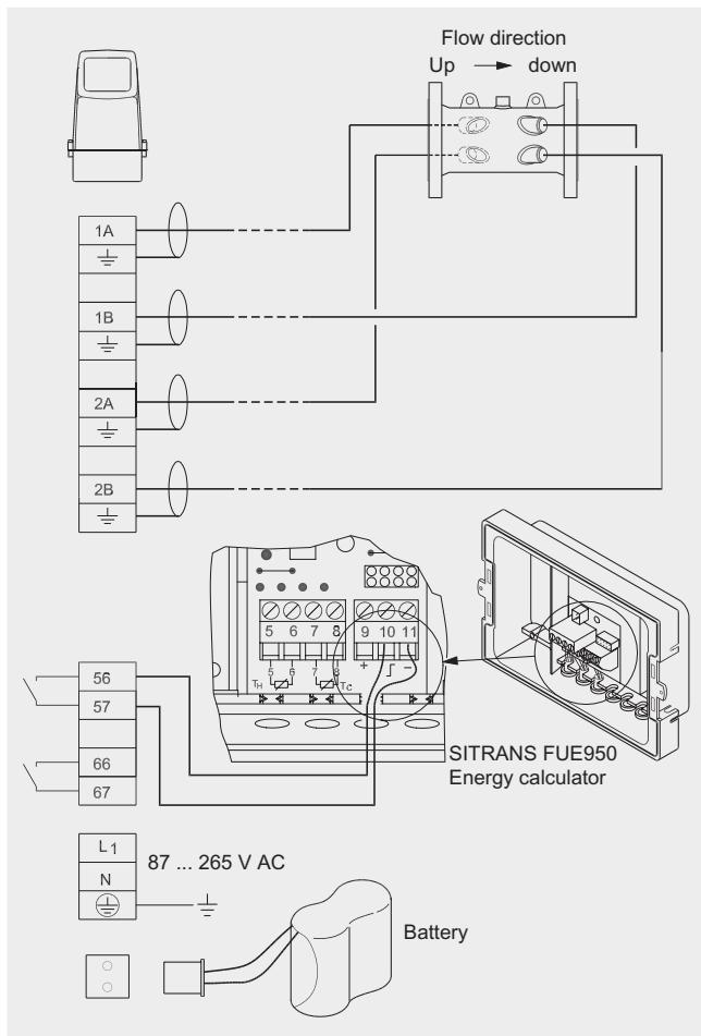
The scheme shows the transducer cable connections between transmitter terminals and respective transducer and the electrical connection of the energy calculator SITRANS FUE950.
