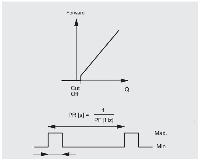
Pulse volume: output A/B configured as volume per pulse, calculated on forward/reverse or net forward/reverse flow. The volume per pulse is free scaleable (via PDM software) if the sealing is open.
