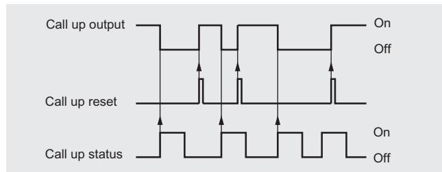
Call up: the call up output is active until manually reset by use of PDM program. The callup function is activated when an alarm is activated.
